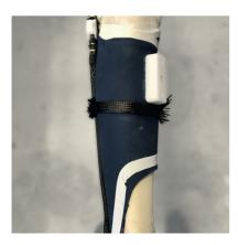
The dummy is glued directly onto the padding so that it is under the first layer of film.
