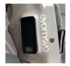
When viewed from the outside, the recess for the cable should now be at the bottom.
