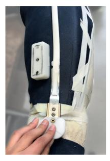
When positioning the dummy, it is important to note that the cable of the evomove® control unit must reach from the lower edge of the dummy to outside the system to enable the plugs to be connected later.
